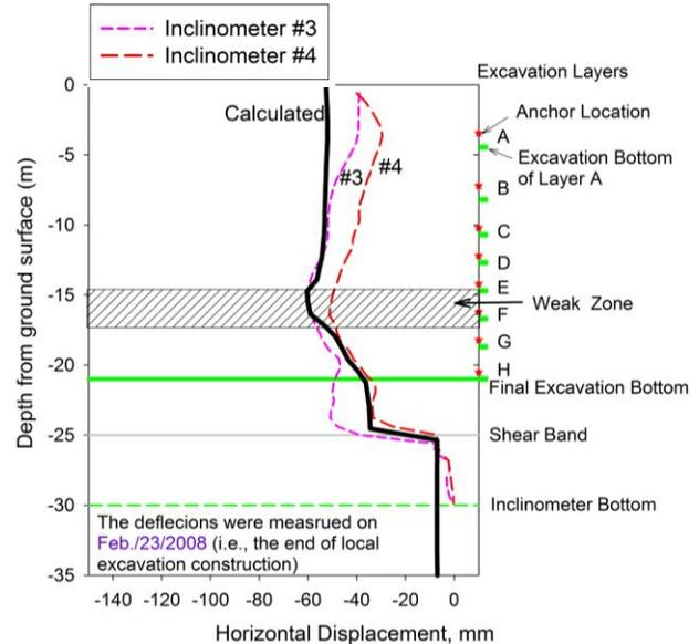
Figure 6. Calculated and measured resultant deflections at #3 and #4 on the north side
