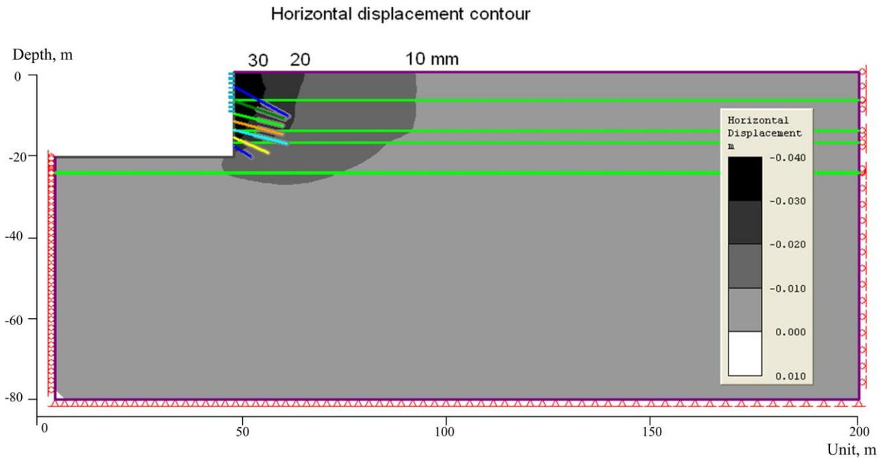
Figure 12b. Horizontal displacement contour (calculated) at #5 and #6
