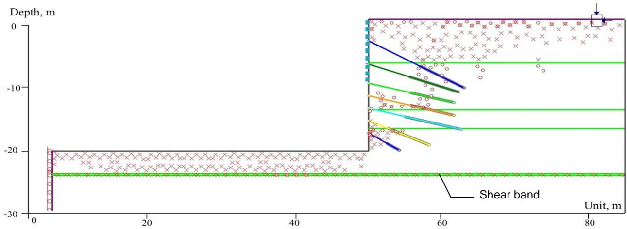
Figure 9. Plastic zone distribution from numerical analysis
