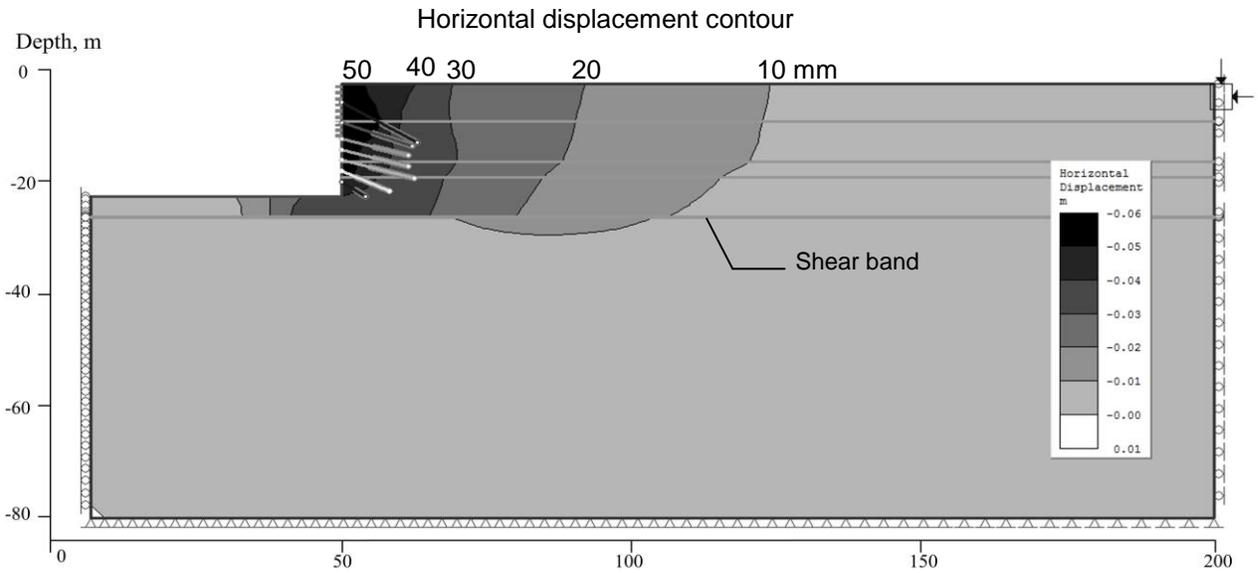
Figure 8. Horizontal displacement contour (calculated)
